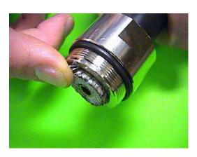
7. Insert the spring finger pin of the forward section of the connector into the center conductor. You should hear a snap. Spin the forward section of the connector clockwise while pushing it against the cable and holding the back section firm.
