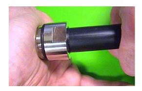
6. At this point you should see from 1/8"-3/16" of braid protruding beyond the gland washer. Make sure that this braid is visible around the entire circumference. The braid should then be spread across the face of the connector
