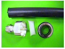
2. Cut the corner of the lubricant packet and apply the lubricant liberally to the O-ring in the aft section of the connector.
