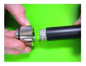
5. Use the palm of your hand to snap the back end of the connector over the jacket.
