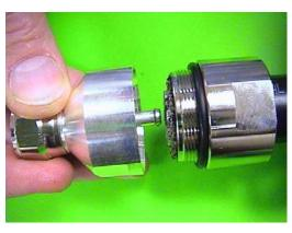
8. Using 1 1/4" open end wrenches, torque the sections together to the point that the Oring between the sections is compressed. Hold the back section firm while spinning the front section.
