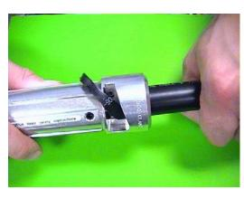
4. Straighten any braid that may have been disturbed during the stripping process. Slide the back section of the connector over the braid without disturbing it. Be sure that the axis of the connector is in line with the axis of the cable.
