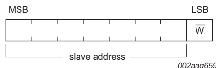
Fig 27. The first byte after the START procedure
