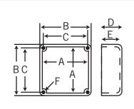
Junction boxes are supplied with threaded brass insert, brass screws, PVC gasketing and mounting feet. Nylon and stainless steel screws, as well as larger sizes of fabricated junctions box, are available upon request. (F = Threaded brass insert size.)
