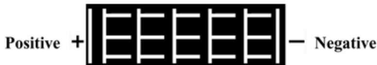
**Warning! Do not connect a charged battery backwards or reverse polarity to the solar module, this will destroy the solar module and may cause the battery to explode causing bodily harm, even death!**
