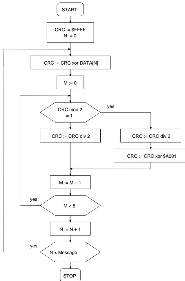
This results in the following calculation for function 48 with device address 250: CRC16\_H= 4, CRC16\_L= 67.
